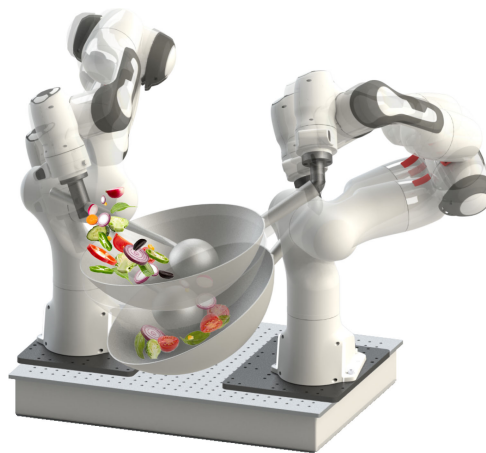
Fig. 1. Robot stir-fry is a non-prehensile manipulation of semi-fluid objects which requires highly dynamic movements and continuous bimanual coordination in a long time series.
