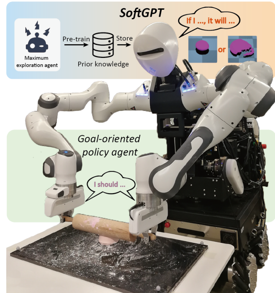
Fig. 1. The proposed pipeline of soft object manipulation contains two parts: a pre-trained SoftGPT model for providing prior knowledge about soft object manipulation and a goal-oriented policy for each specific task.
